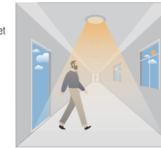
The sensor turns light ON when motion gets detected.
